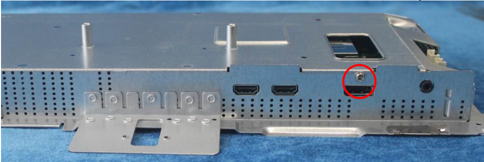
S7. Turn over the shield and unscrew the screws on main board and power board.
